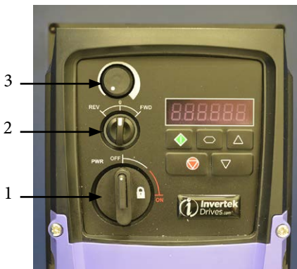
Fig. 1 Pump operation switches
