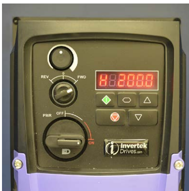
Fig. 4 Switch 3 set to 200 Hz
