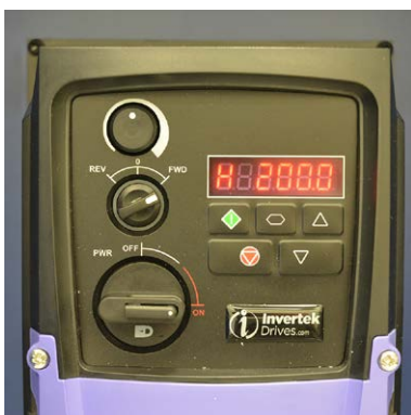
Fig. 8d Switch 3 set to 200 Hz
