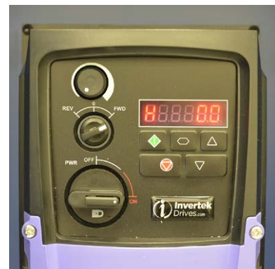
Fig. 8c Switch 2 set to FWD
